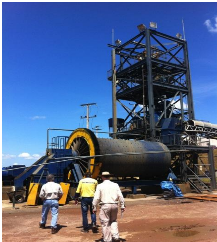
Figure 1. Ball Mill and Gravity Tower at Cleveland's Premier Mine in Goiás, Brazil.
