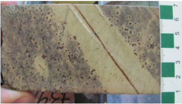
Wongoni Project Drillhole DD92HV14 - 75m Pyrite-iron oxide veining with intense albite alteration selvage in silica-sericite- haematite altered volcaniclastic
