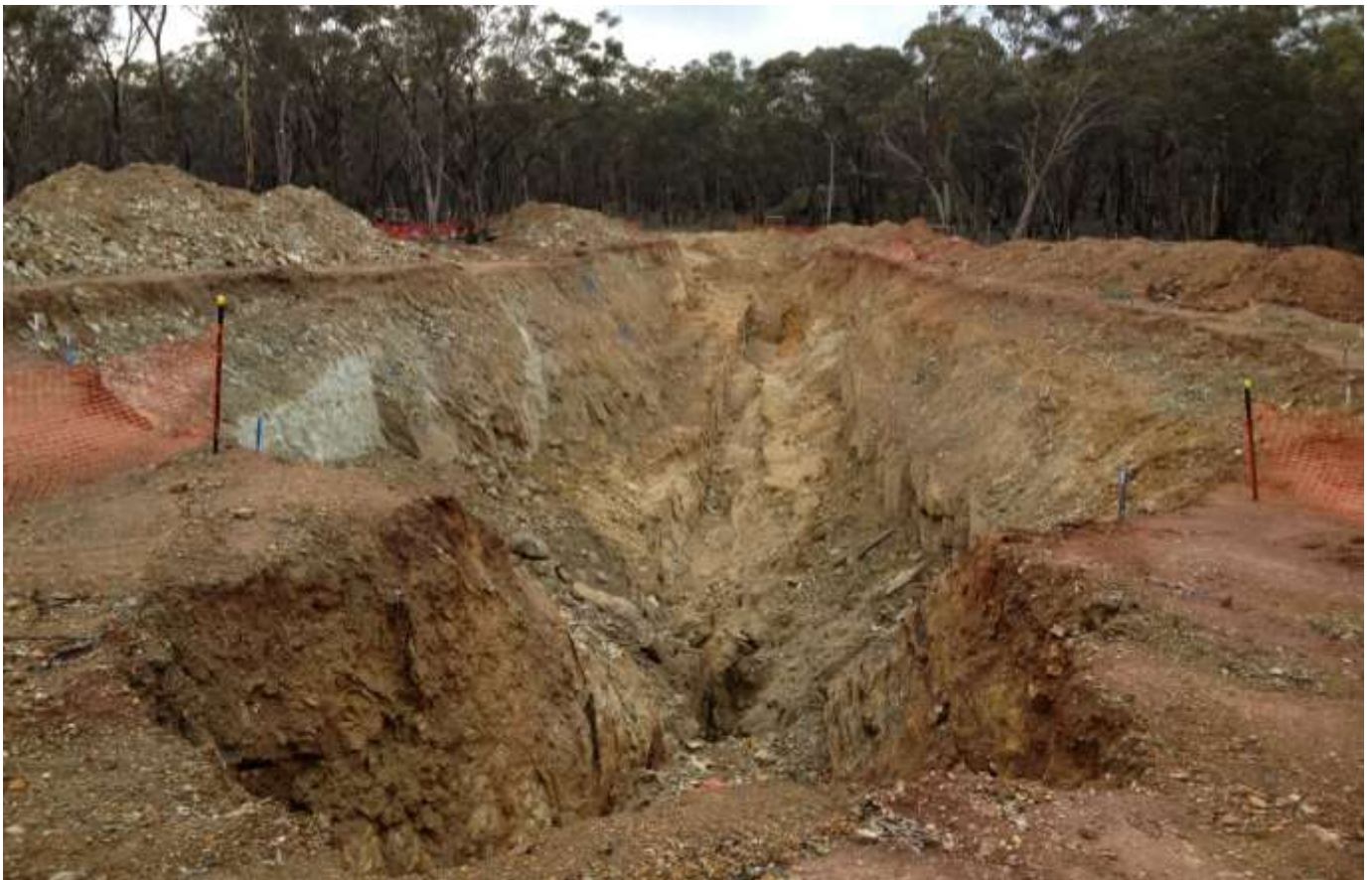
Black Reef Stage 1 open pit mined to 15 metres depth
