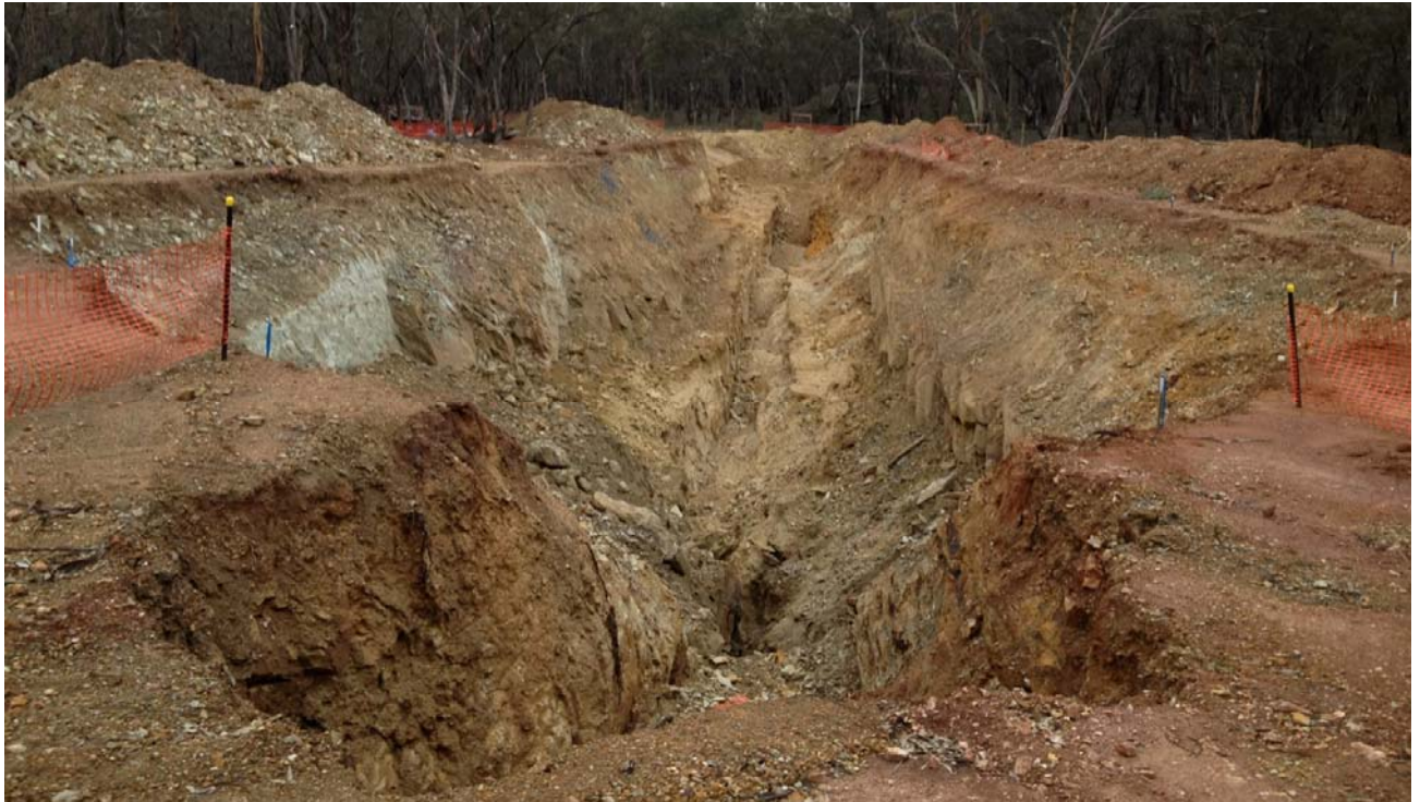
Black Reef Stage 1 open pit mined to 15 metres depth (view north)
