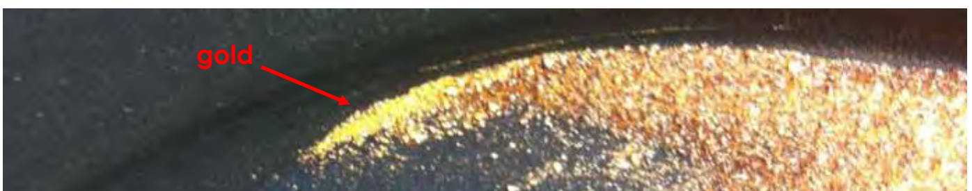
Gold tail in gold pan from sample FRR019 20-21 metres (assay result: 138.8 g/t Au)
