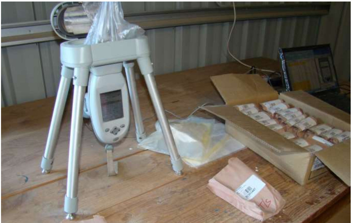
Analysis of aircore drilling pulp samples using a Niton XLt 500 Series Portable XRF Analyser
