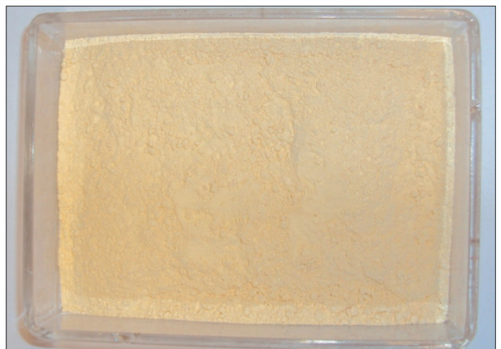
Photo 1: High purity (99.9%) rare earth oxide product produced from Ngualla mineralisation by the SX Pilot Plant at ANSTO Minerals.
