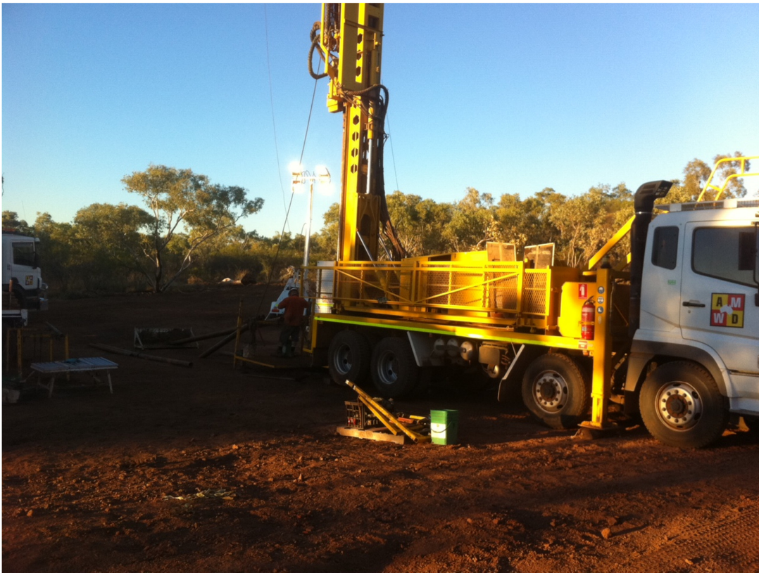
Figure 1: Diamond drill hole LBD4 in progress
