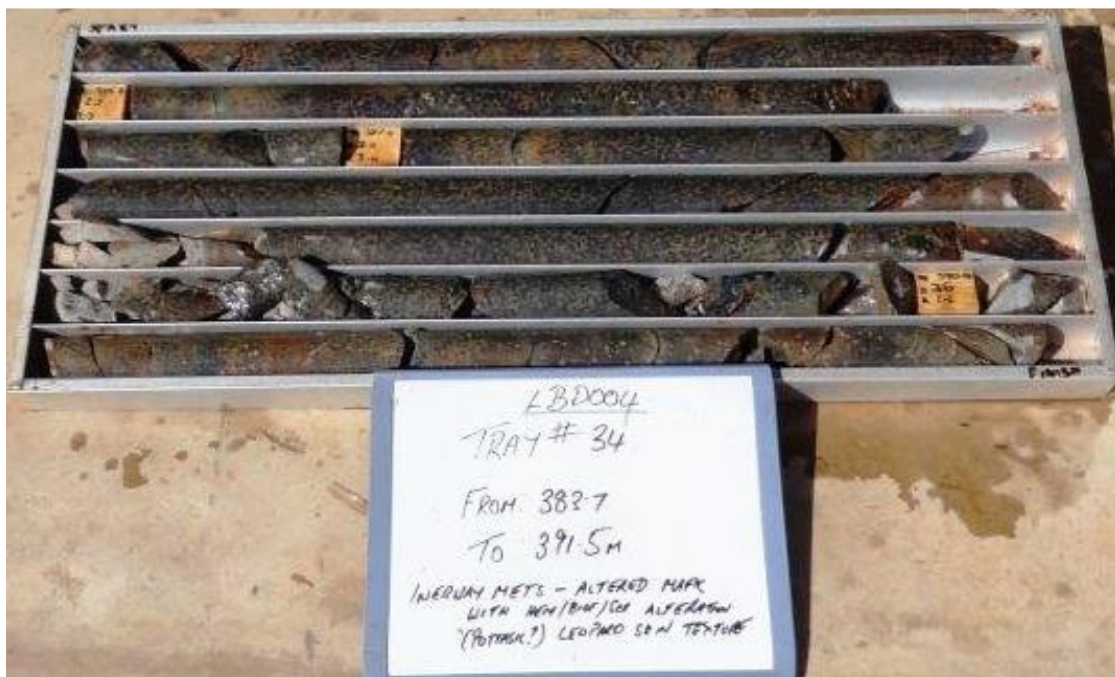
Figure 7. Leopard spot" textured intrusive rock unit suggestive of possible fine-grained Gabbro composition
