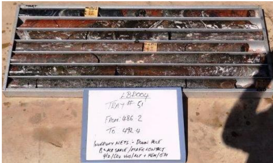
Figure 6. Pervasive quartz-carbonate-haematite development in black shale and mafic rock
