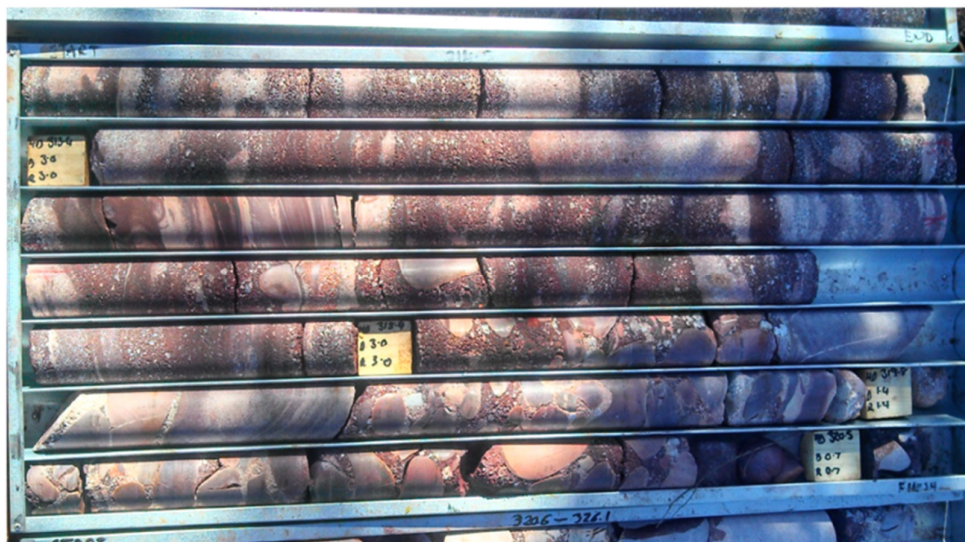
Figure 2. Limbunya Formation basal unconformity, sandstone-conglomerate rock to 326m depth.
