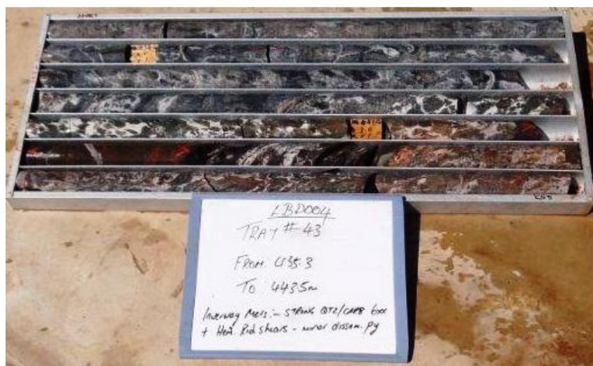
Figure 4. Strong quartz-carbonate-haematite development (hydrothermal-alteration of mafic rock).
