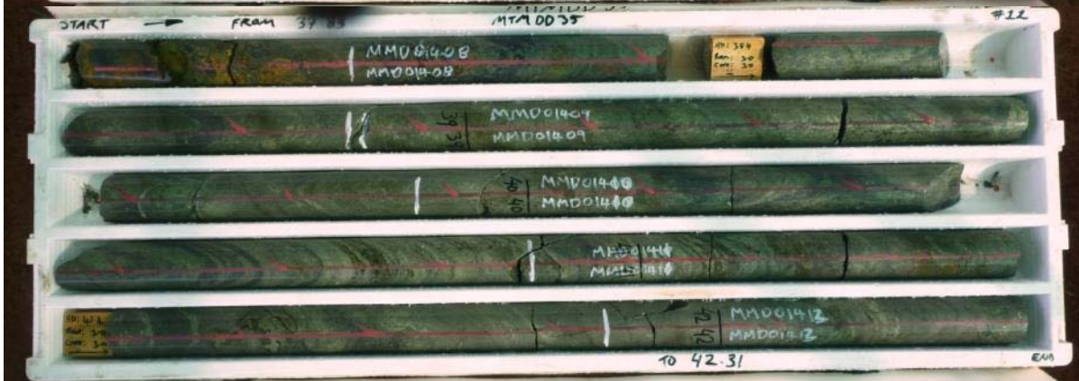
MTMDD35 – core containing Massive Sulphide and Stringer Sulphide zones
