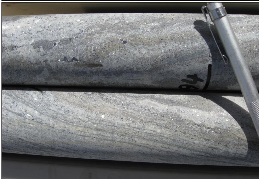
[Figure 4] Maronan Project: Typical strong visible lead sulphide mineralisation from fresh banded carbonate-lead sulphide rock in MRN12003B at 1234.3 metres down hole (above) and MRN12004B at 970.5m (middle) and 994.0m (bottom) down hole. The dominant grey-silver mineral is lead sulphide (galena).
