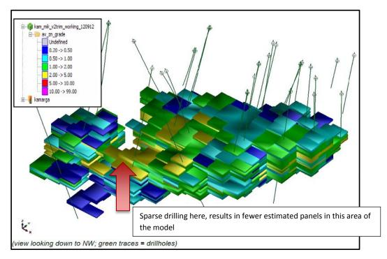
Figure 3 Plan view of resource estimate panels showing average zinc grade for the whole panel
