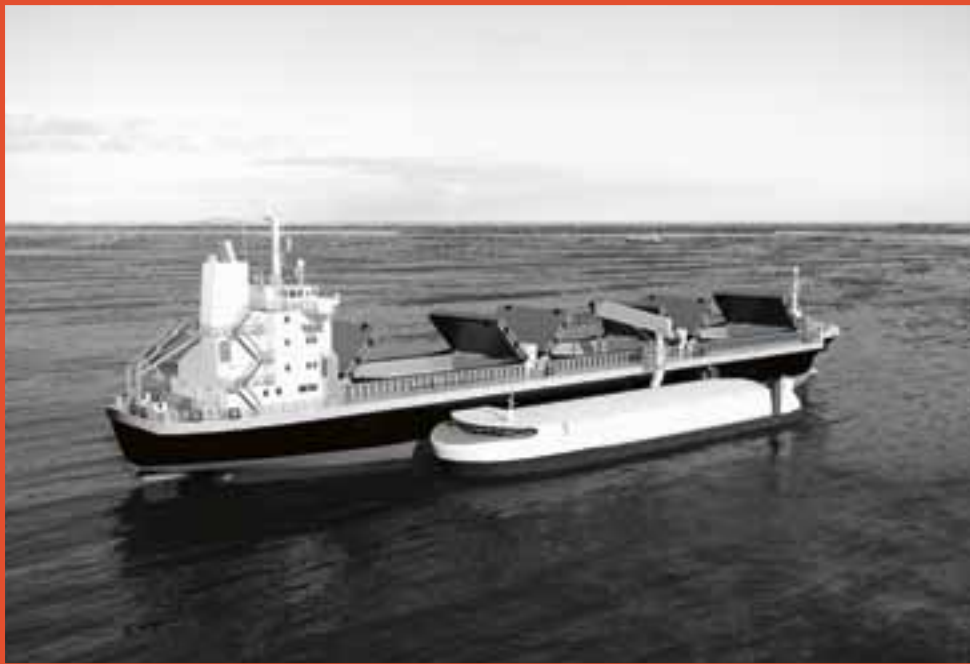
Schematic of self-propelled, self-unloading transshipping barge discharging into offshore ocean going vessel.
