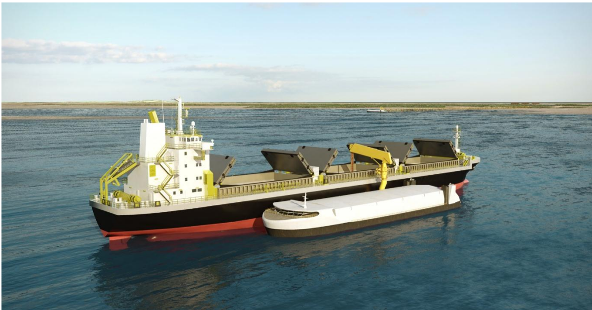
Figure 2.7. Schematic of barge attached to a ship, unloading magnetite concentrate.
