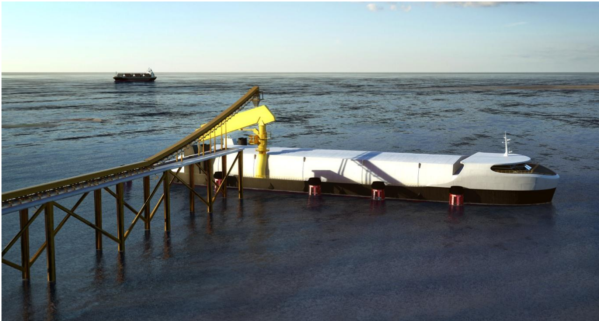
Figure 2.6. Schematic of self powered, self unloading barge at the end of the jetty
