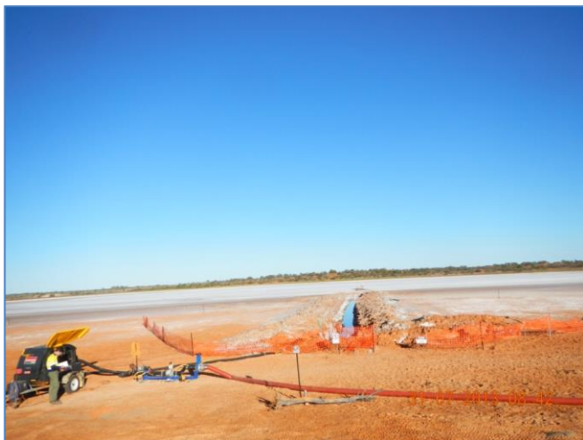
Pump test in progress and discharge pipe at Pulcura Lake Trench.
