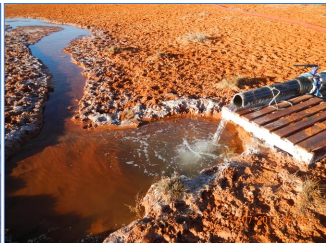
Pump test in progress and discharge pipe at Pulcura Lake Trench.
