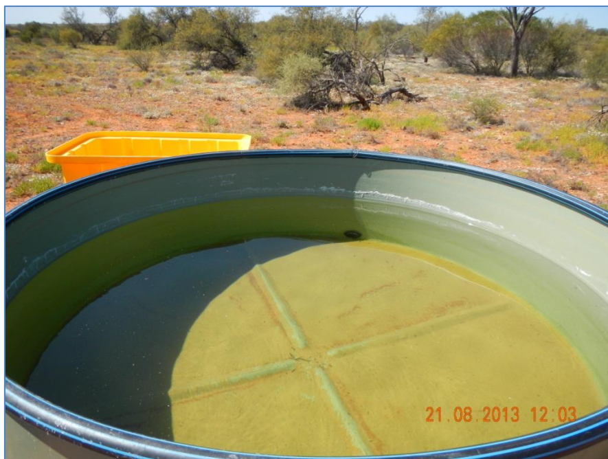
Tank 3 Evaporation trial on August 21 with salt crystals visible around the rim.
