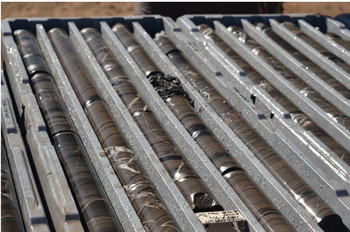
Figure 5: Trays of high grade laminated/bedded zinc sulphide (brown colour) from hole TNDD009
