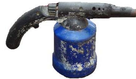
Unauthorised blowtorch Heat generated: 800 deg C
