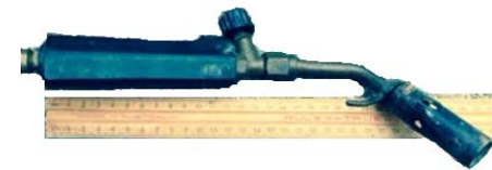
Standard issue blowtorch equipment Heat generated: 450 deg C
