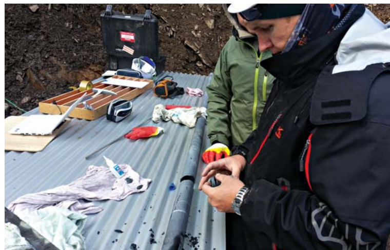
Diamond core inspection.
