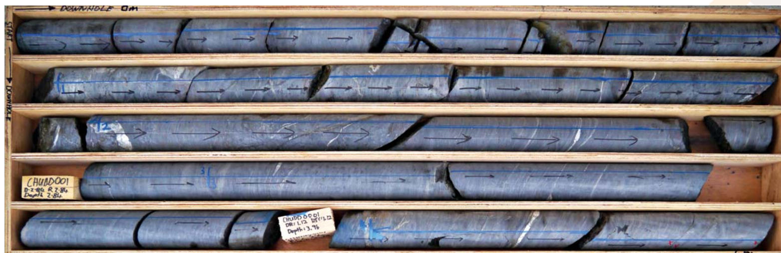
Figure 2: First core box from the 2013 Chubu drilling programme showing hanging wall slate units.
