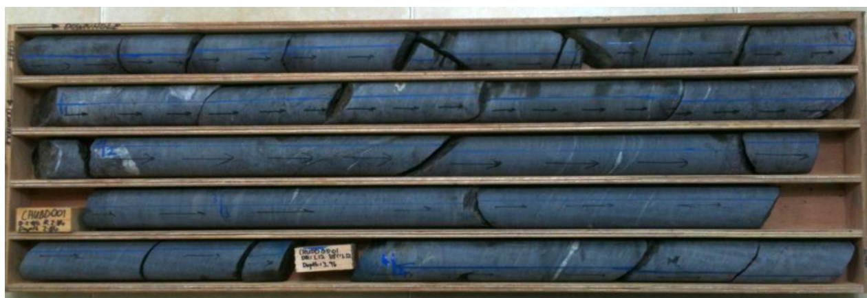
Figure 4: First core box from the 2013 Chubu drilling program showing hangingwall slate units
