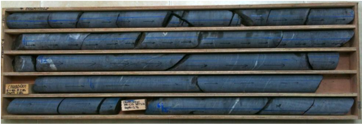
Figure 10: First core box from the 2013 Chubu drilling programme showing hanging wall slate units
