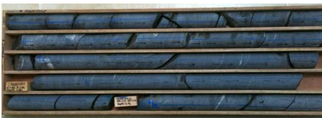
Figure 4: First core box from the 2013 Chubu drilling programme showing hanging wall slate units
