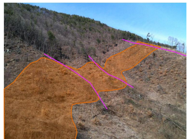
Figure 6: Location of three completed trenches (magenta line) at Chubu during March 2013 and location of mapped uranium and vanadium mineralised black shale. Note: Some trenches have been extended beyond the boundaries of the mapped black shale where strong vanadium mineralisation persists into hangingwall and footwall units. The co-existence of Uranium and Vanadium will enable a production process which will
