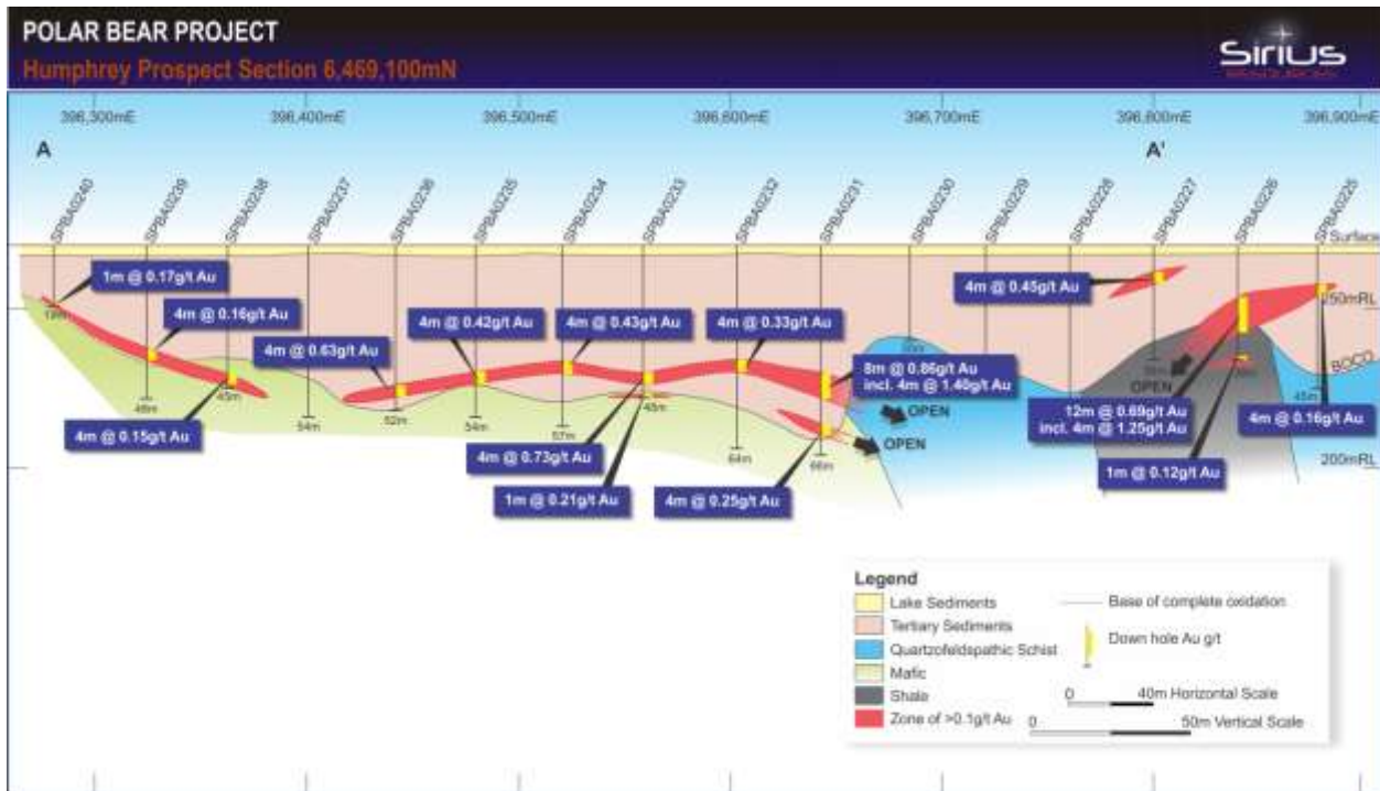
Figure 3: Lake Cowan aircore drilling program, Au distribution line 6,469,100mN.
