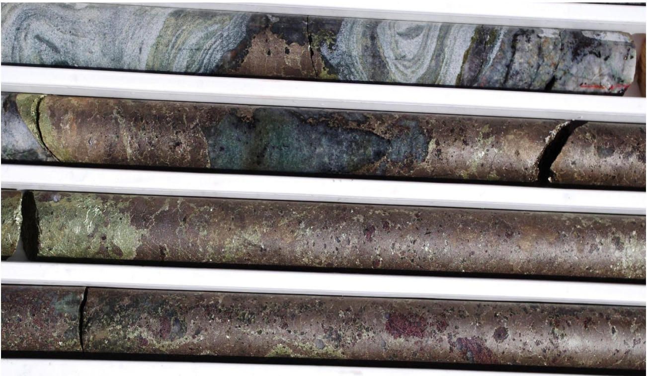
Figure 3. Photo of breccia sulphide from SFRD0251, showing fragments of wallrock, large red garnet crystals, the pale banded carbonate (marble) marker bed, brassy yellow clots of chalcopyrite (copper), silvery crystals of pentlandite (nickel) and bronze coloured pyrrhotite.
