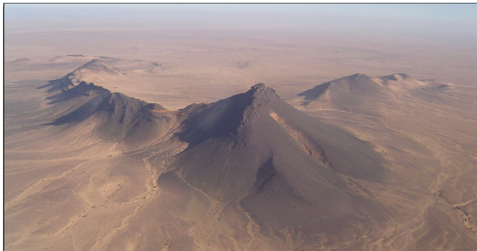
Figure 3: Guelb el Aouj East deposit looking north Showing the southern closure, western and eastern limbs of the synform structure
