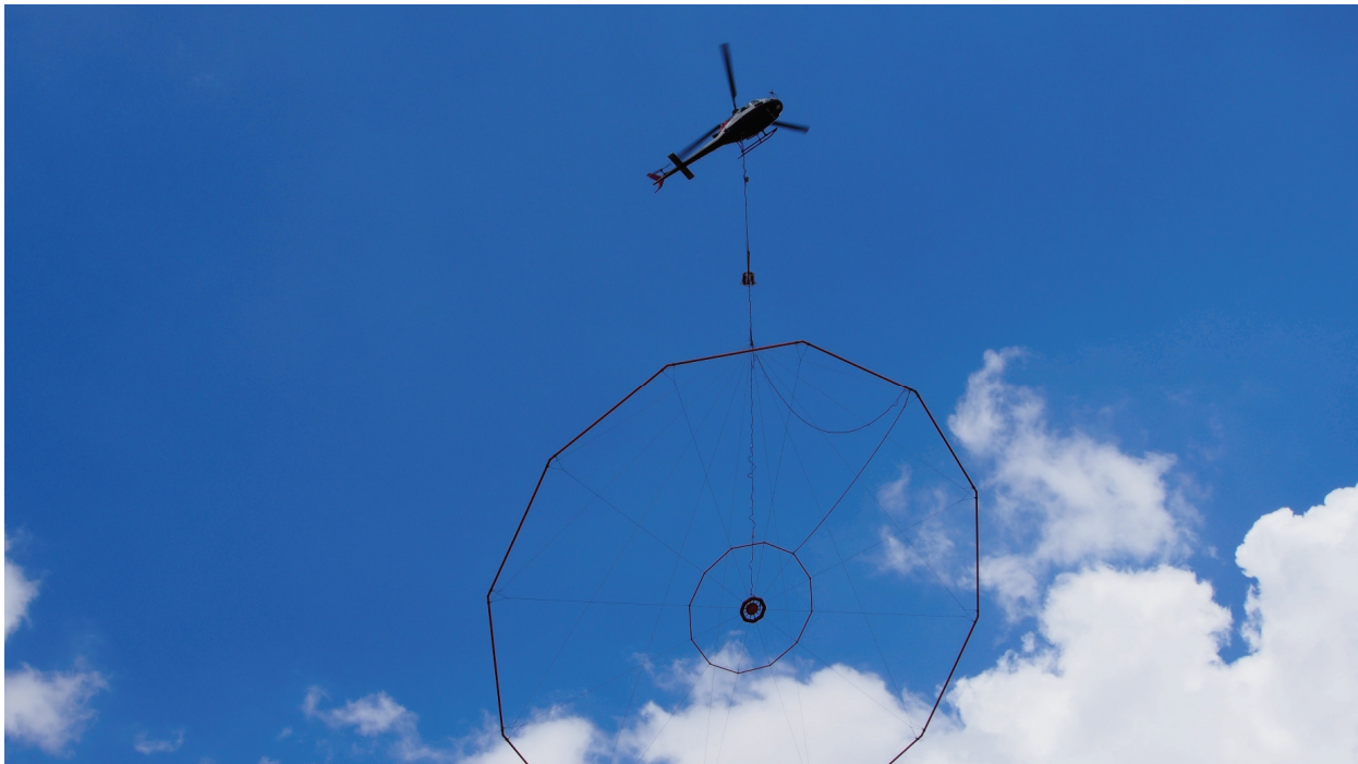
Figure 5. HeliVTEM system in action over the Duwi area.
