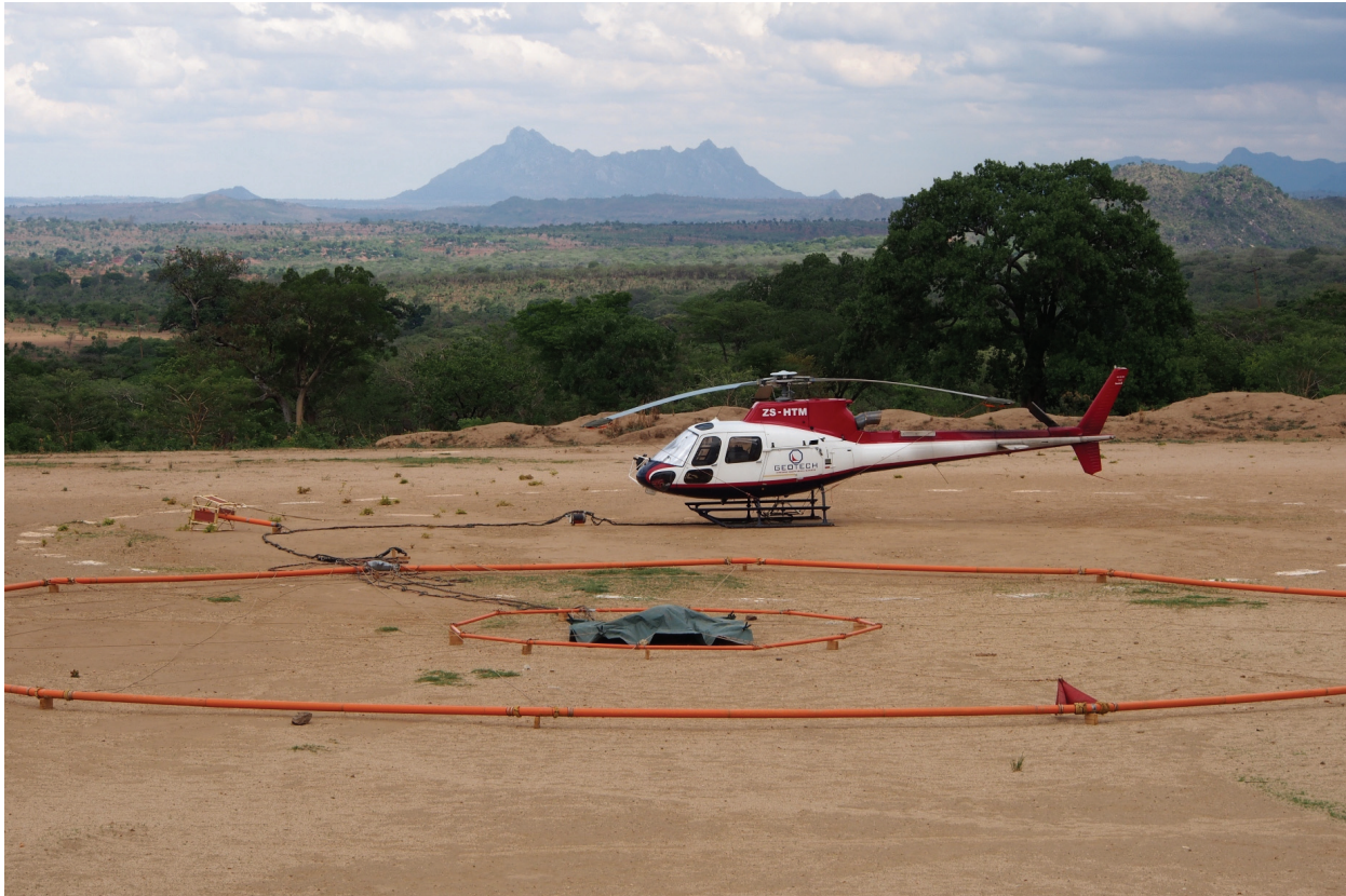
Figure 4. HeliVTEM system ready for flight. View looking east from Lilongwe over the greater Duwi area.
