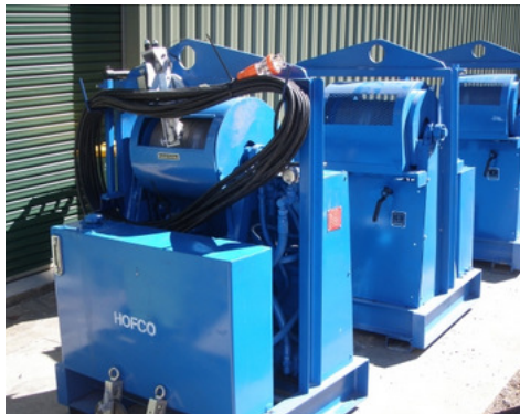
Wire Line Unit
