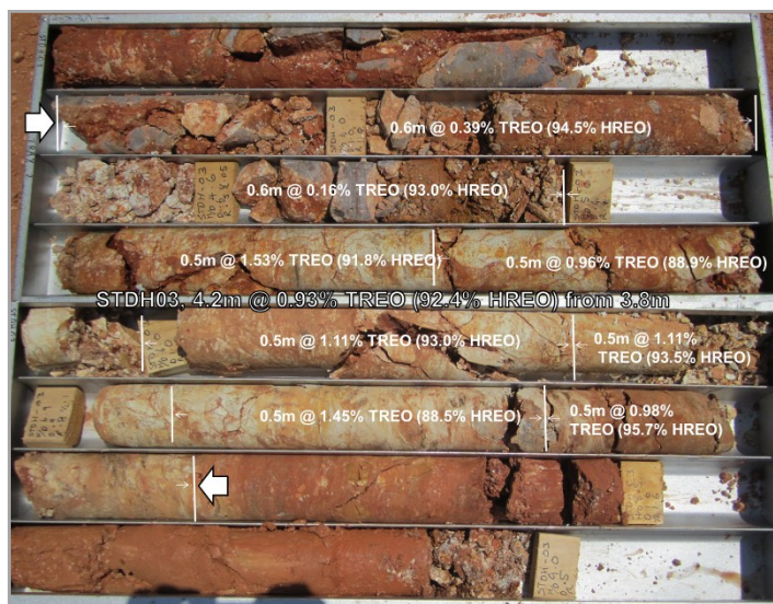
Figure 2: Drill core STDH3 showing significant intersection and clay host rock types similar to Southern China Clay Hosted Rare Earth Deposits.
