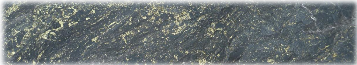
THDD236 – disseminated chalcopyrite in a graphitic shale, 405m down hole.
