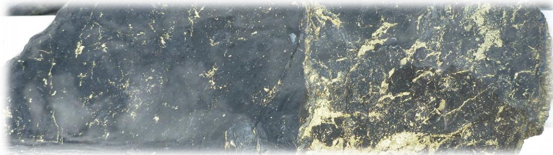
THDD236 – disseminated and vein chalcopyrite in a graphitic shale, 391m down hole.
