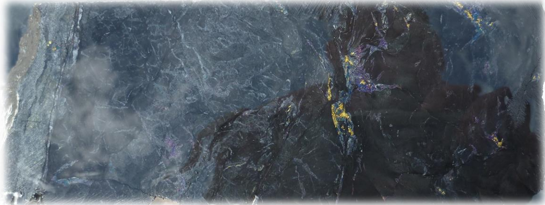
THDD238 – chalcocite replacing bornite replacing chalcopyrite in a graphitic shale, 573m down hole.
