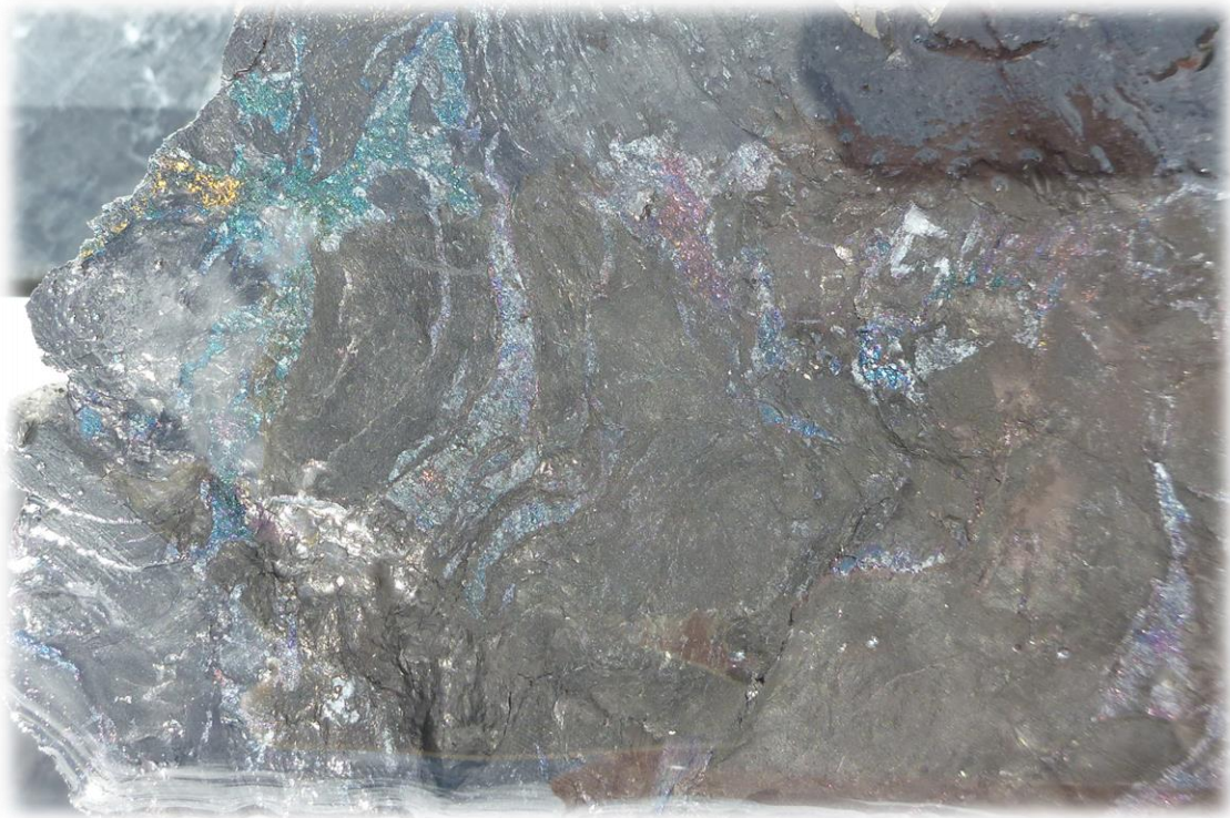
THDD235 – disseminated and vein bornite in a graphitic shale, 616m down hole.
