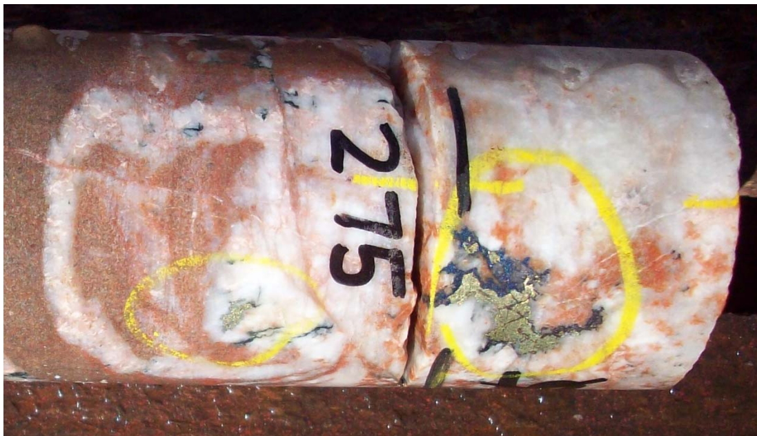
BIF Hill prospect - Chalcopyrite and bornite mineralisation observed in quartz veining at BIF Hill hole 12BH003 (275m depth)
