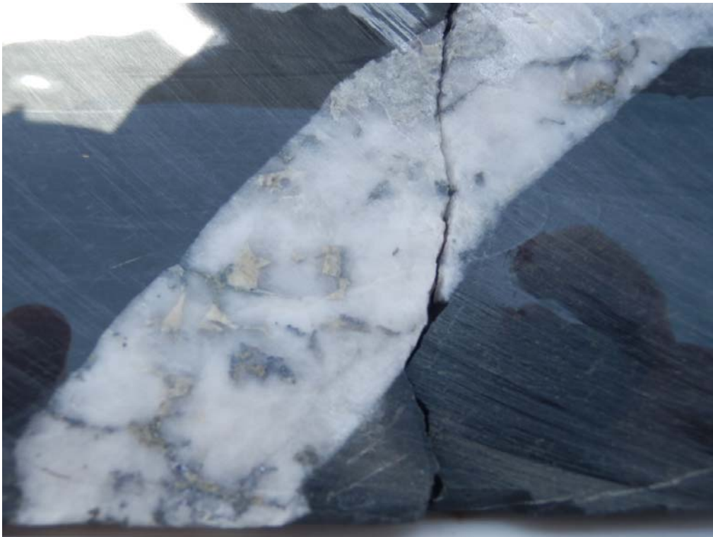
Spring Hill project – Diamond drill core with quartz vein containing visible gold.
