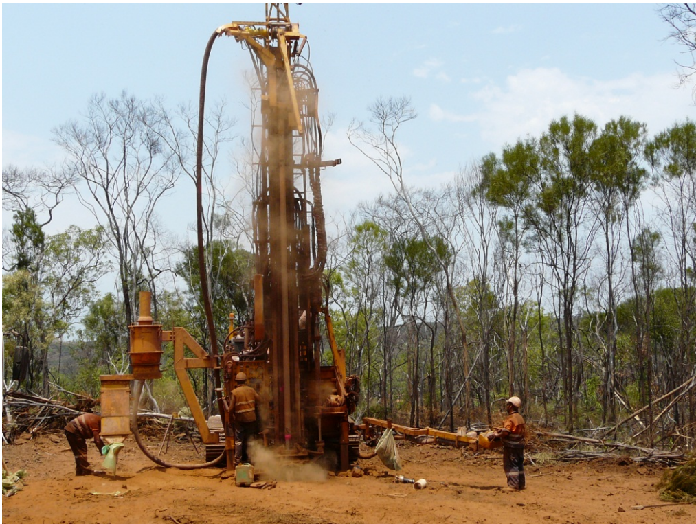
Mountain Creek project - Reverse Circulation drill rig.
