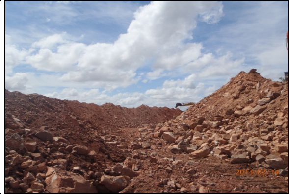
Stockpiled crusher feed material for concrete aggregate
