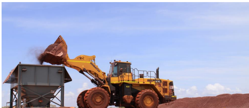
Fig 2: Loading of stockyard bin conveyor system at Bing Bong Loading Facility (BBLF).
