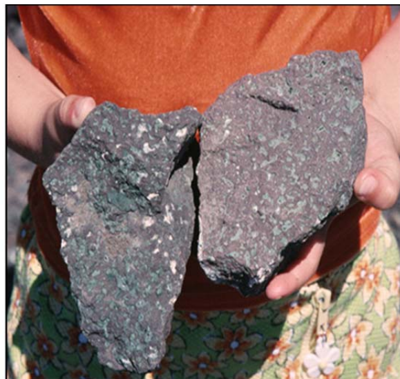
Photo of lava (amygdaloid) samples from Keeweenaw Peninsular, Michigan Copper. Producer of 15 billion pounds of copper metal between mid 1800's and 1990.
