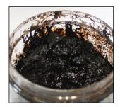
The SSF method involves exposing an organic solvent extract of <63 micron soils to ultraviolet light. The extract will emit radiation back at wavelengths corresponding to mono and ployaromatic hydrocarbons that are present in high, medium and low gravity crude oil.
