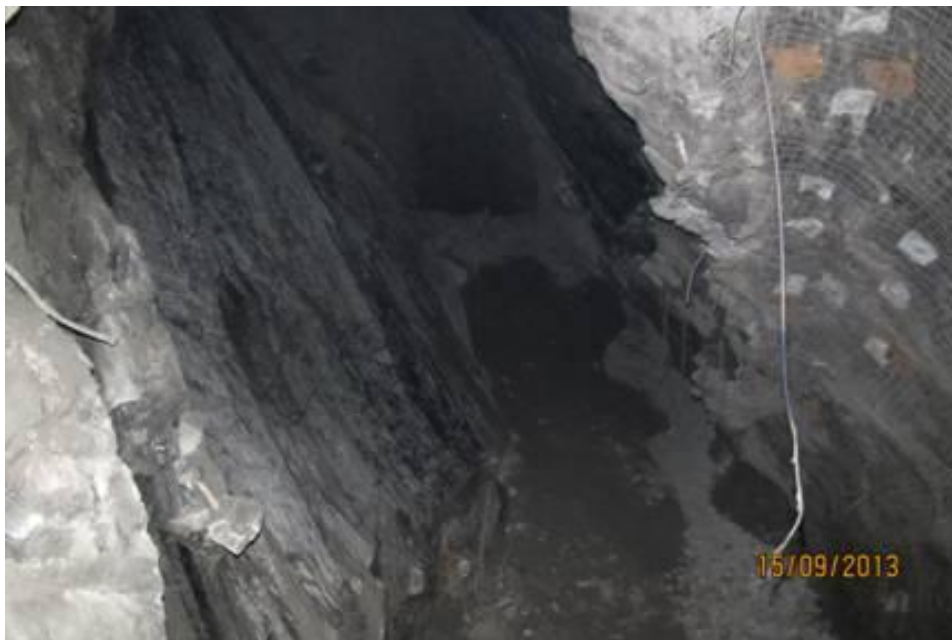
1110 Panel 4 longhole stope void prior to paste filling
