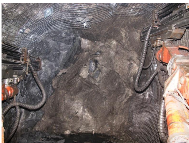
Flying Fox 285 South Ore Drive face showing massive sulphides @ 5.0% nickel
