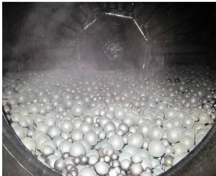
Cosmic Boy Concentrator ball mill showing the grinding media charge
