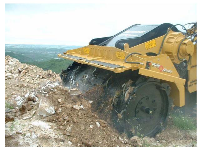
Figure 3: Vermeer Surface Miner: Close-Up of Cutter Wheels
