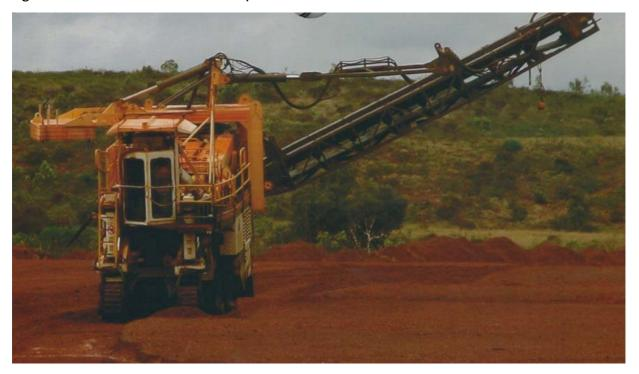
Figure 4: Wirtgen Surface Miner
