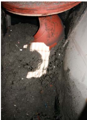
Fig 5: Organic fraction post Wet Density Separation conveyed into bioconversion vessel V1 (March 2014).
