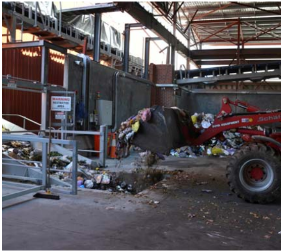
Fig1: Municipal solid waste (MSW) loaded onto trommel (March 2014).
