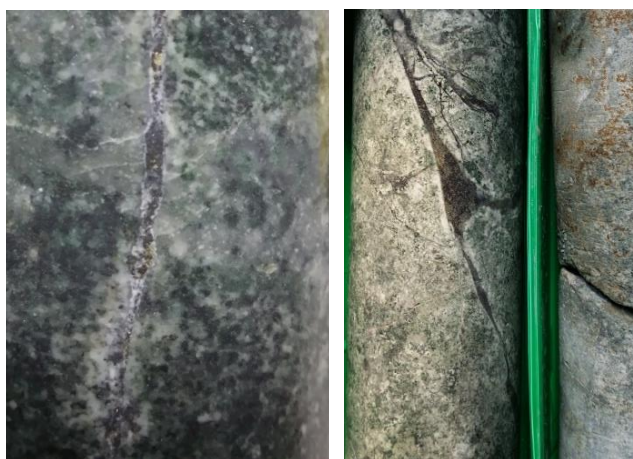
Photos of TRDD055 drill core at 154-m (left) and 174-m (right) down-hole Altered diorite intrusion cut by porphyry-style quartz-magnetite-pyrite-anhydrite veinlets containing traces of chalcopyrite & molybdenite mineralisation
