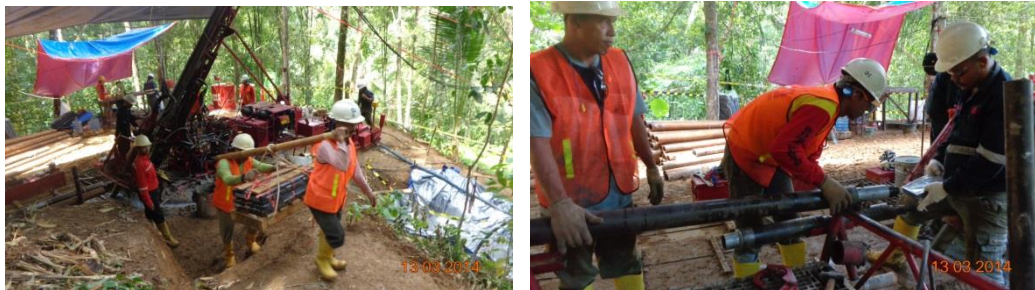
Singgahan Prospect – Maxidrill MXD-420 man-portable rig drilling TRDD055
