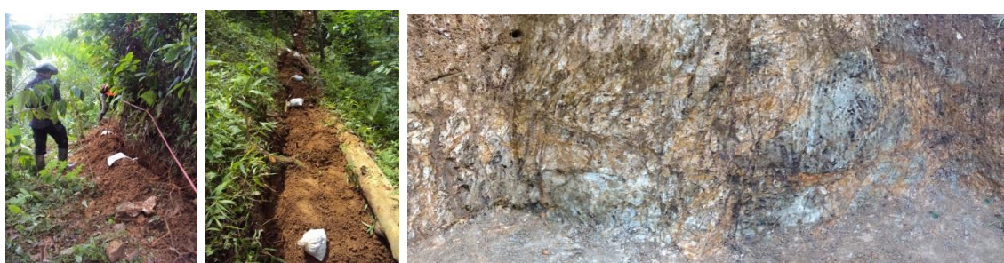
Singgahan Prospect – Contour benching & limonitic quartz stockwork exposed in diorite
