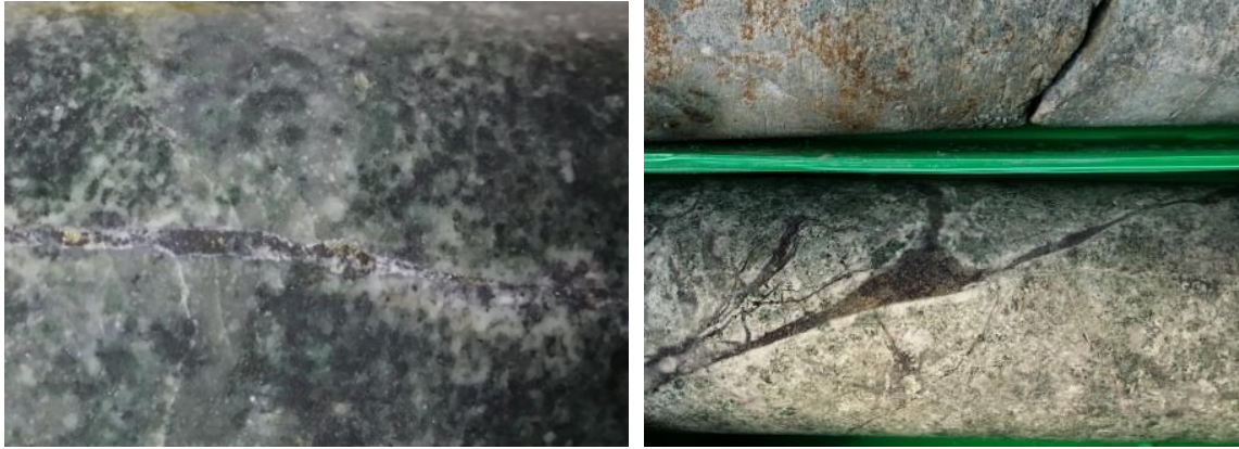
Singgahan Prospect – TRDD055 HQ drill core Quartz-magnetite-anhydrite-pyrite veined & altered diorite containing traces of disseminated chalcopyrite & molybdenite
