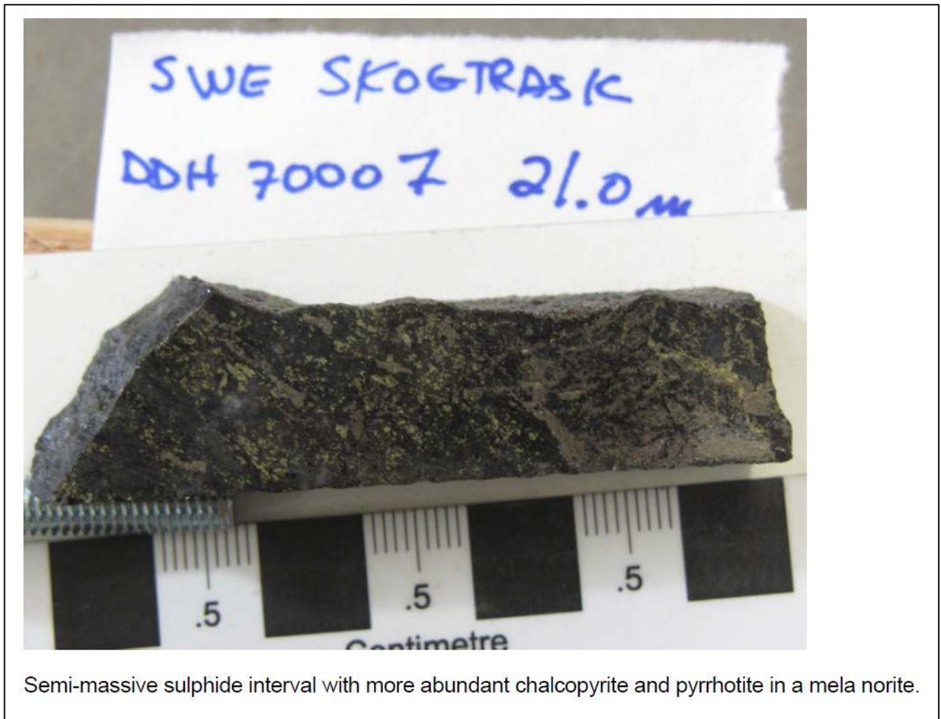
Figure 6. Portion of the core sampled from DDH 7007 over the interval 20.8 to 21.53m. The interval assayed 0.3 % Nickel and 0.5 % Cu (see Table 2 for the assays for the complete mineralised interval for hole DDH 7007)
