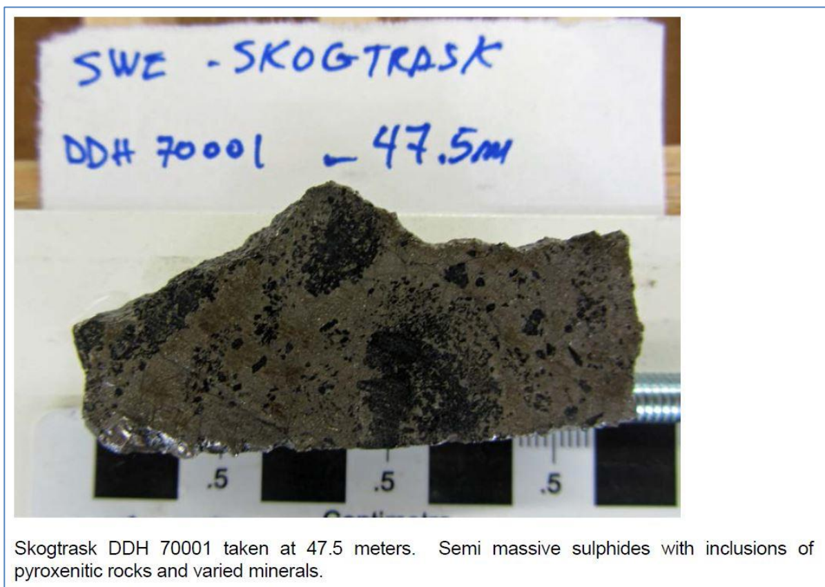
Figure 5. Portion of the core sampled from DDH 7001 over the interval 46.3 to 48.3m. The interval assayed 1.1% Nickel and 0.2 % Cu.
