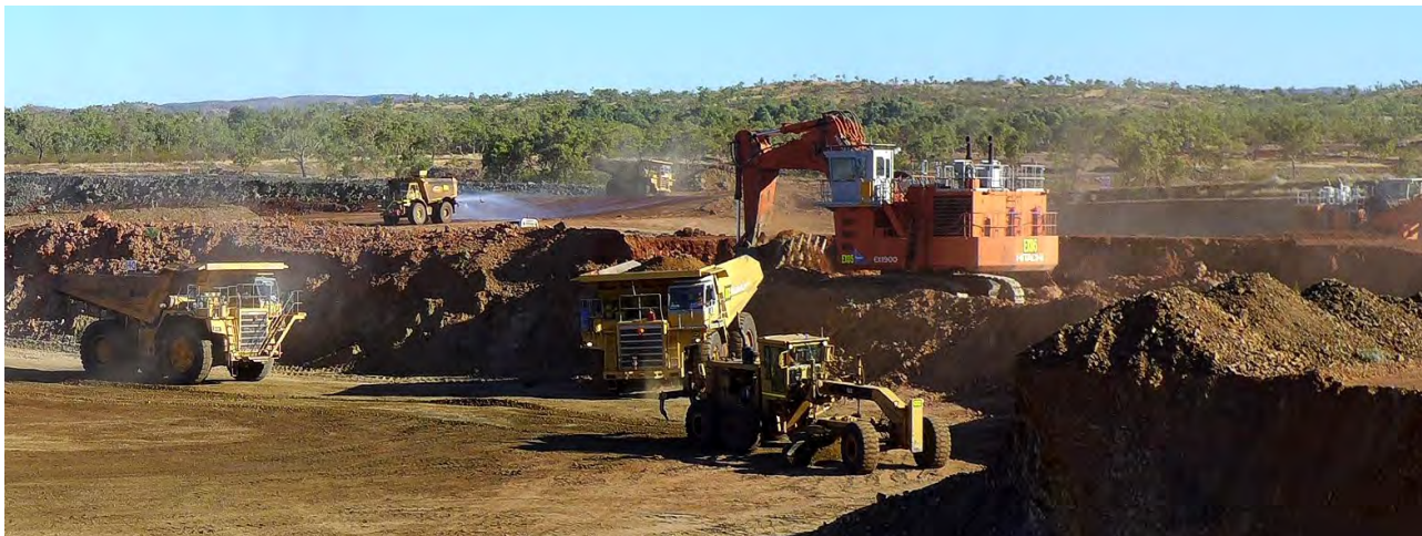
Figure 11: Mining is concurrently underway at the north-west of the LM3 Pit (Final pit), accessing ore and waste previous blasted and remaining in-situ.
