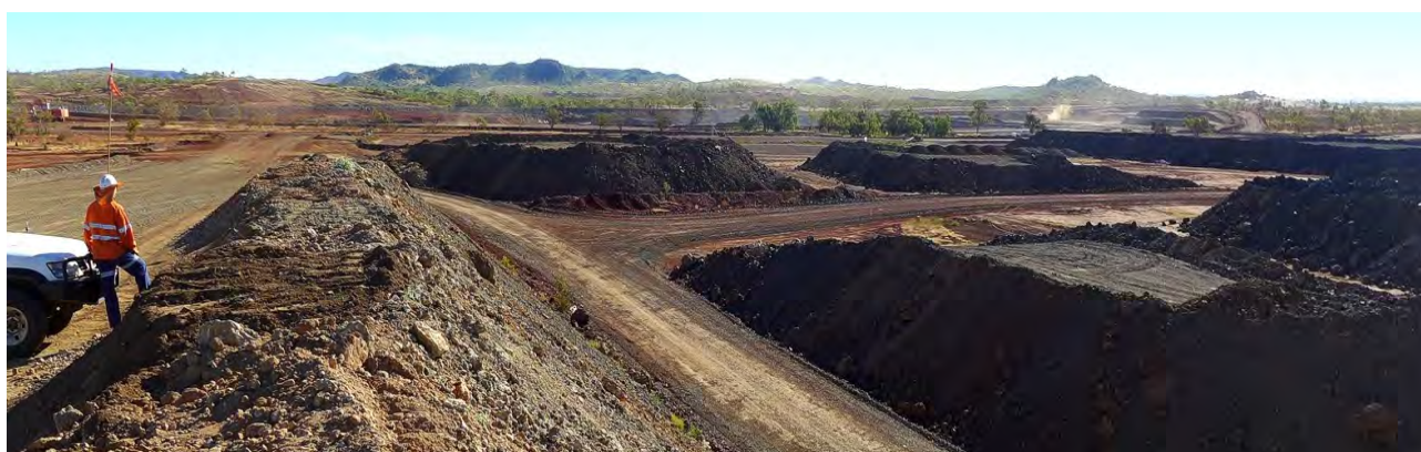
Figure 12: ROM and Stockpile Manager oversees every load of ore and waste coming form the pit to ensure mining losses are kept to a minimum and ore-type segregation remains optimal for the process plant recovery regime. Just one load of high-grade ore accidentally sent to waste can represent over $100,000 of lost metal value to the project. With well over 400 truck-loads removed from the pit every day (soon to increase) a 2% mining loss equates to 8 truck loads a day of lost or poorly reconciled ore...or some 240 trucks per month representing ~22,000 tonnes of lost ore to the project.
