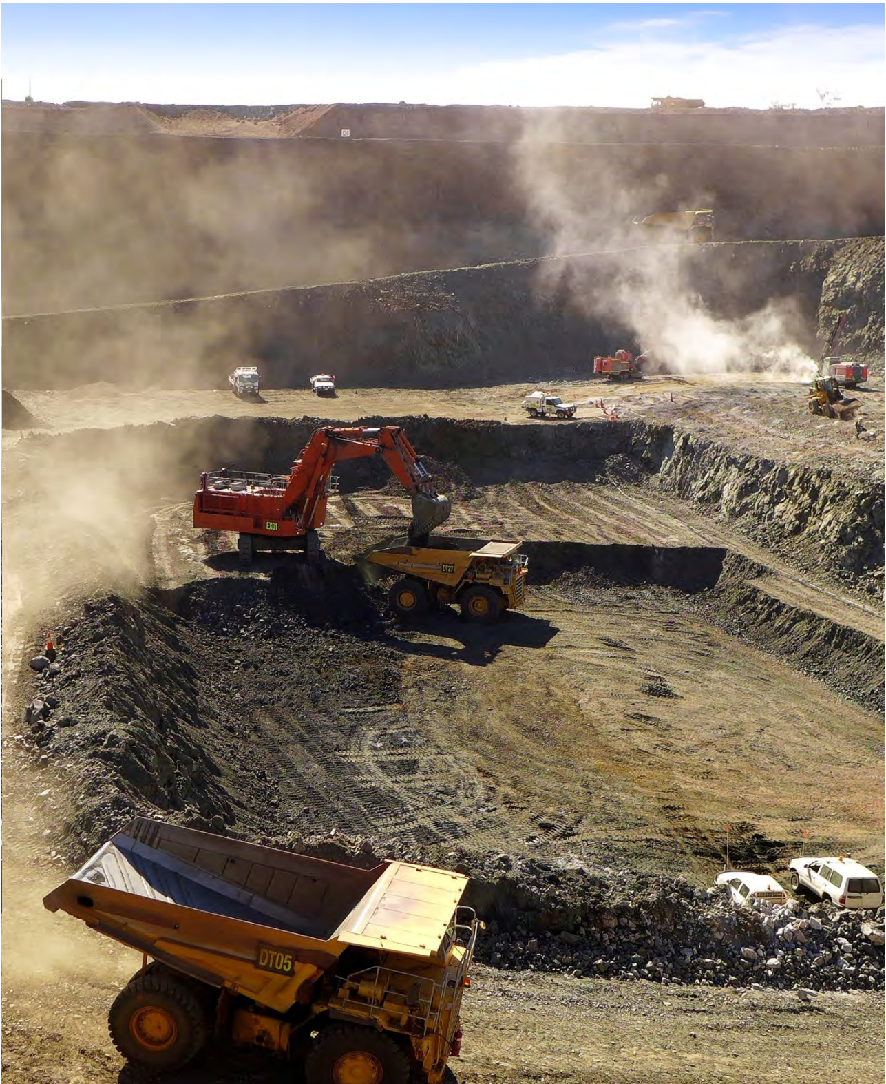
Figure 10: Mining of the very high-grade native copper ore in the LM1 Pit (foreground) as the next blast is loaded (right background). Whilst the truck under the digger is being loaded, another truck arrives (foreground ramp) and the previously loaded truck exits via the background ramp fully loaded. At surface, the truck loaded prior to that is heading to the stockpiles. This cycle continues all day, with 4 trucks per digger ensuring maximum cycle efficiencies.
