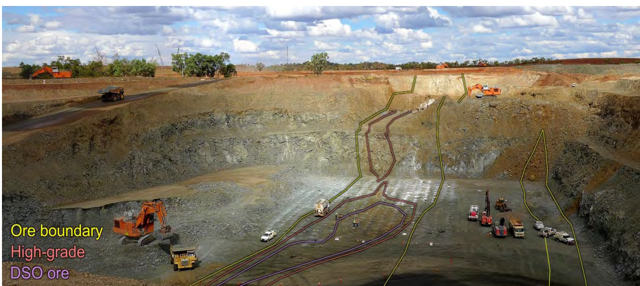
Figure 6: LM1 Pit with indicative ore outlines shown - high-grade native copper ore suitable for DSO is highlighted.
