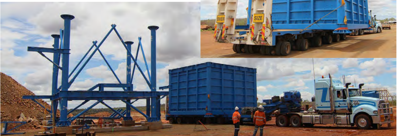
Figure 20: High Pressure Grinding Rolls (HPGR) Surge Bin - at 8m x 10m in footprint, it posed a challenge to ship from Townsville.
