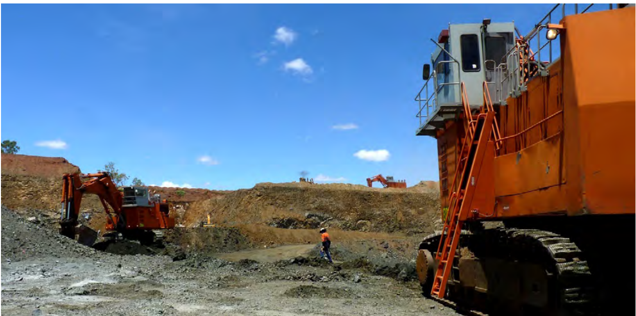
Figure 9: Three diggers (2 in ore) in the LM1 Pit - geologist grade control spotting during a shift change-over
