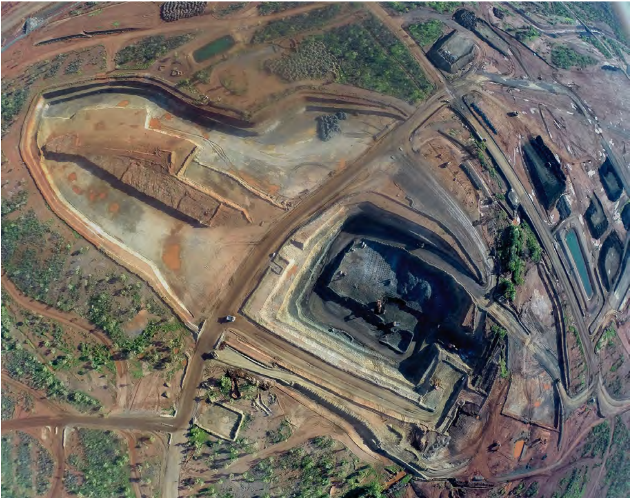
Figure 15: Aerial view showing stage-1 LM1 Pit in the middle of the larger and final LM3 Pit outline. The edge of the stockpile area can be seen to the right.
