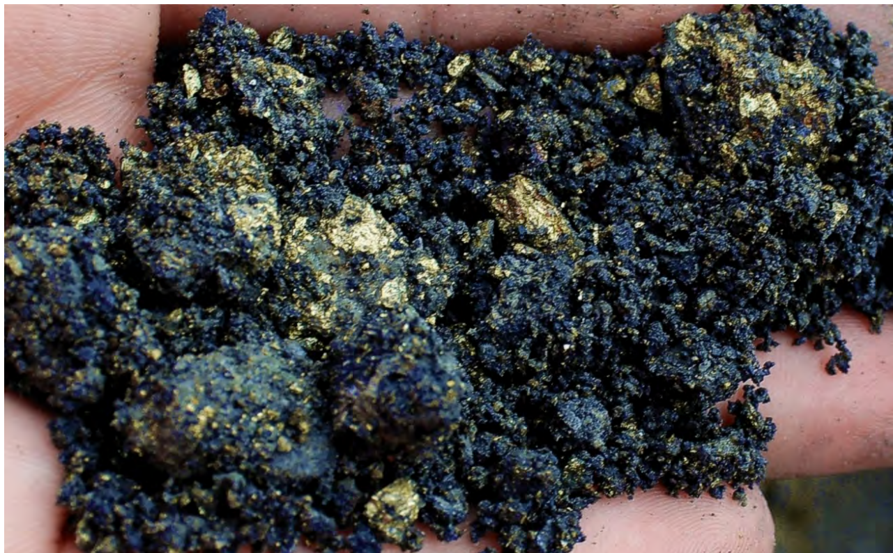
Figure 31: Example of chalcocite rich clays co-mingled with chalcopyrite and resembling the consistency of soil, with copper grades ranging between 24-56% Cu from 30 random XRF spot-checks in the pit.
