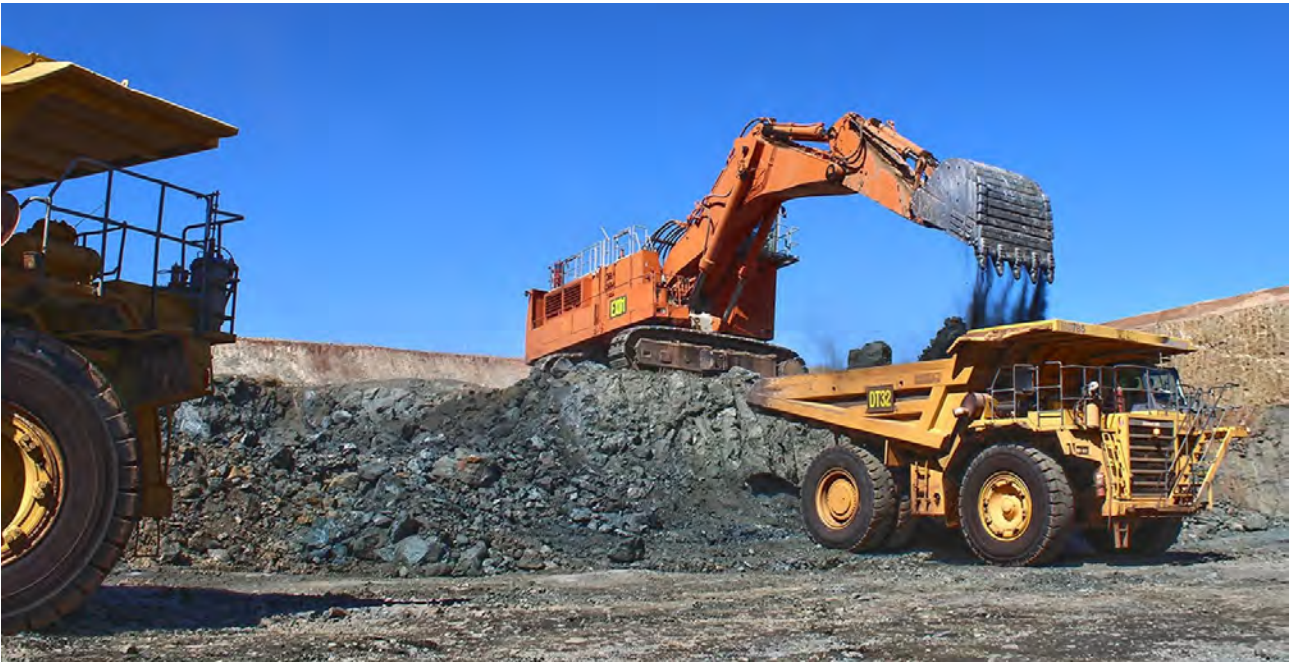
Figure 10: High-grade chalcocite ore being loaded into a dump truck whilst the next truck waits.
