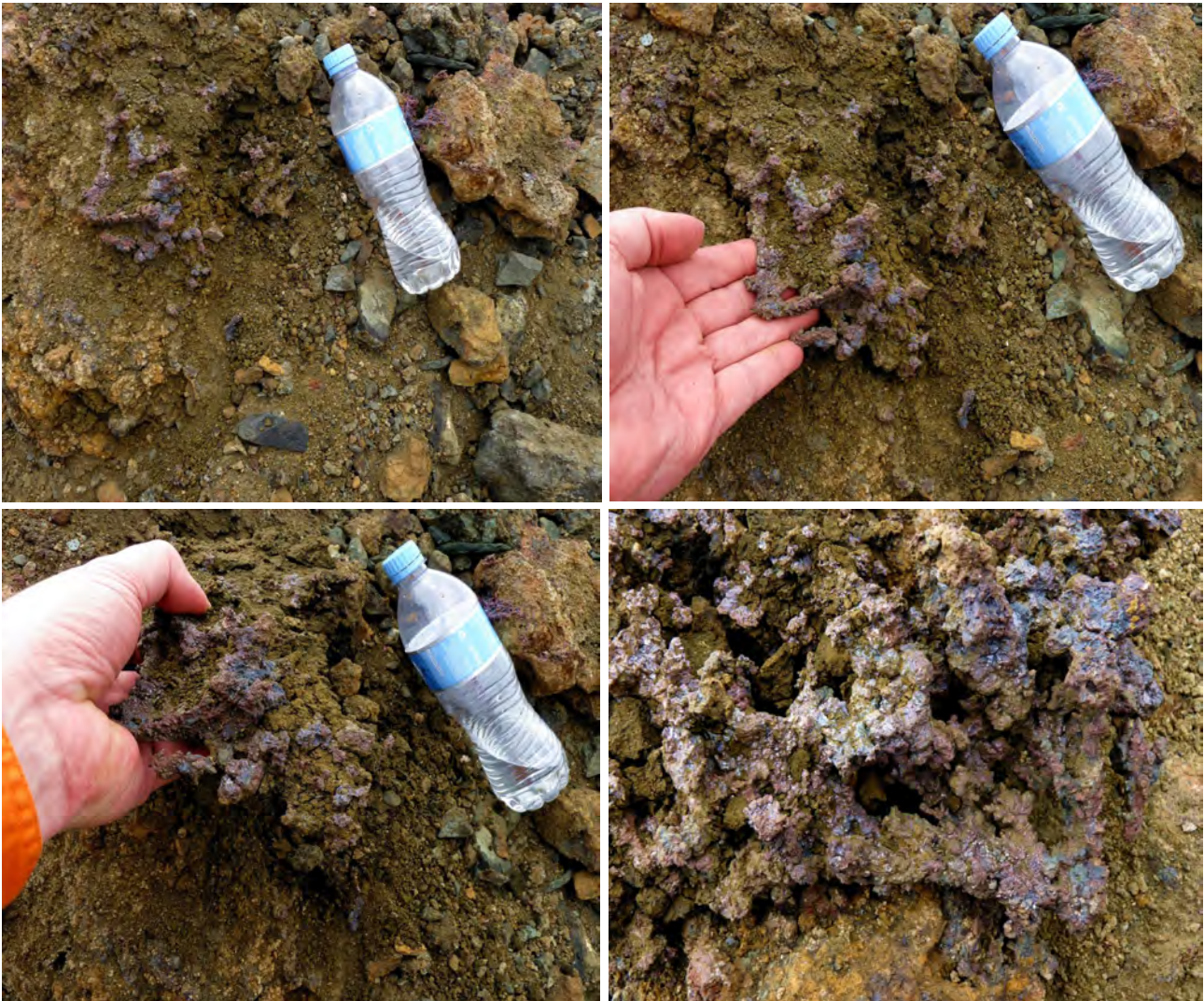
Figure 13: Example of high-grade native copper ore in soft friable matrix (green clays) in Las Minerale (LM1) pit. Image sequence shows ease of pulling native copper nuggets by hand from the ore/rock-face whilst still in-situ.
