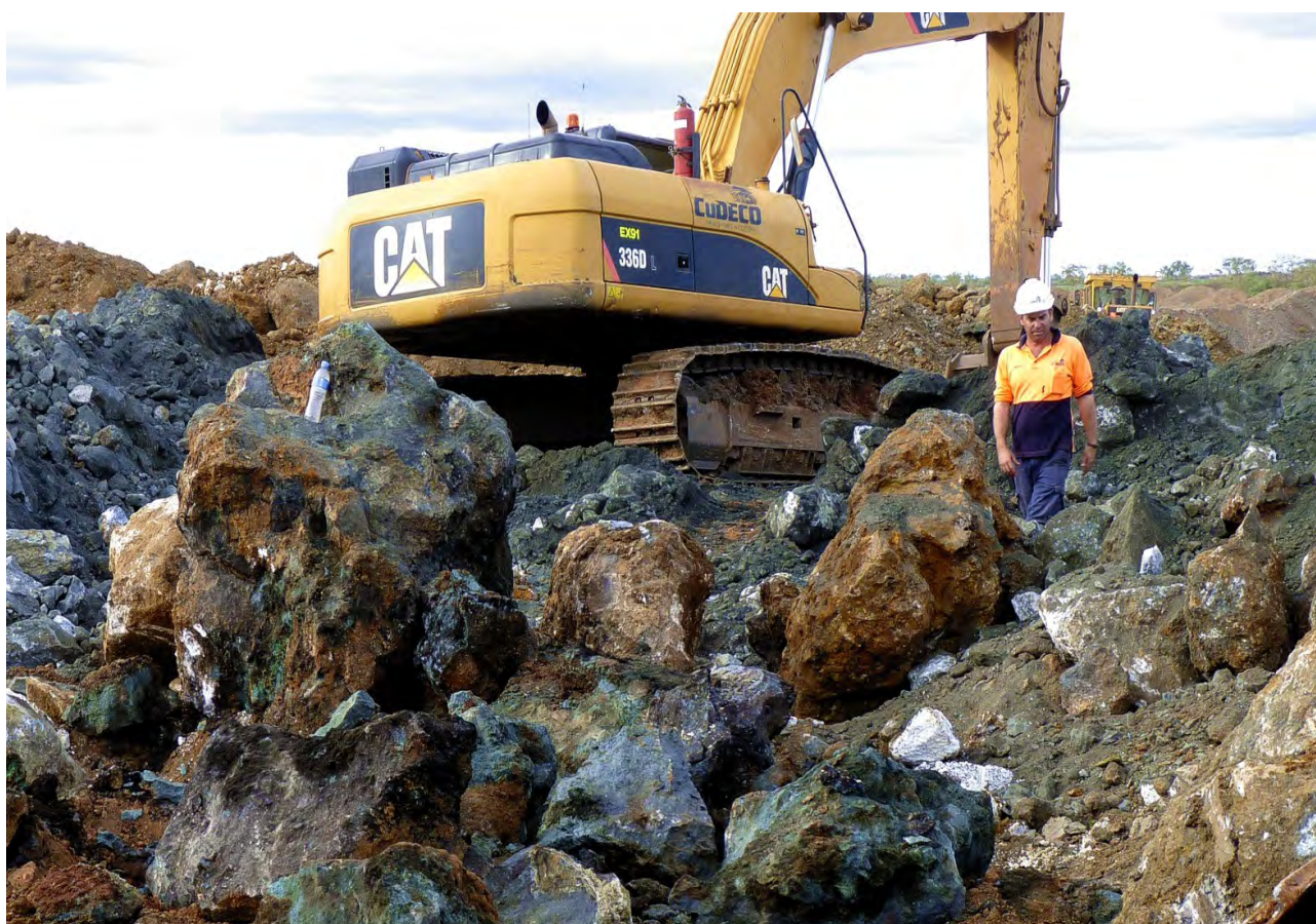
Figure 11: High-grade copper ore being prepared for crushing with rock-breaker
