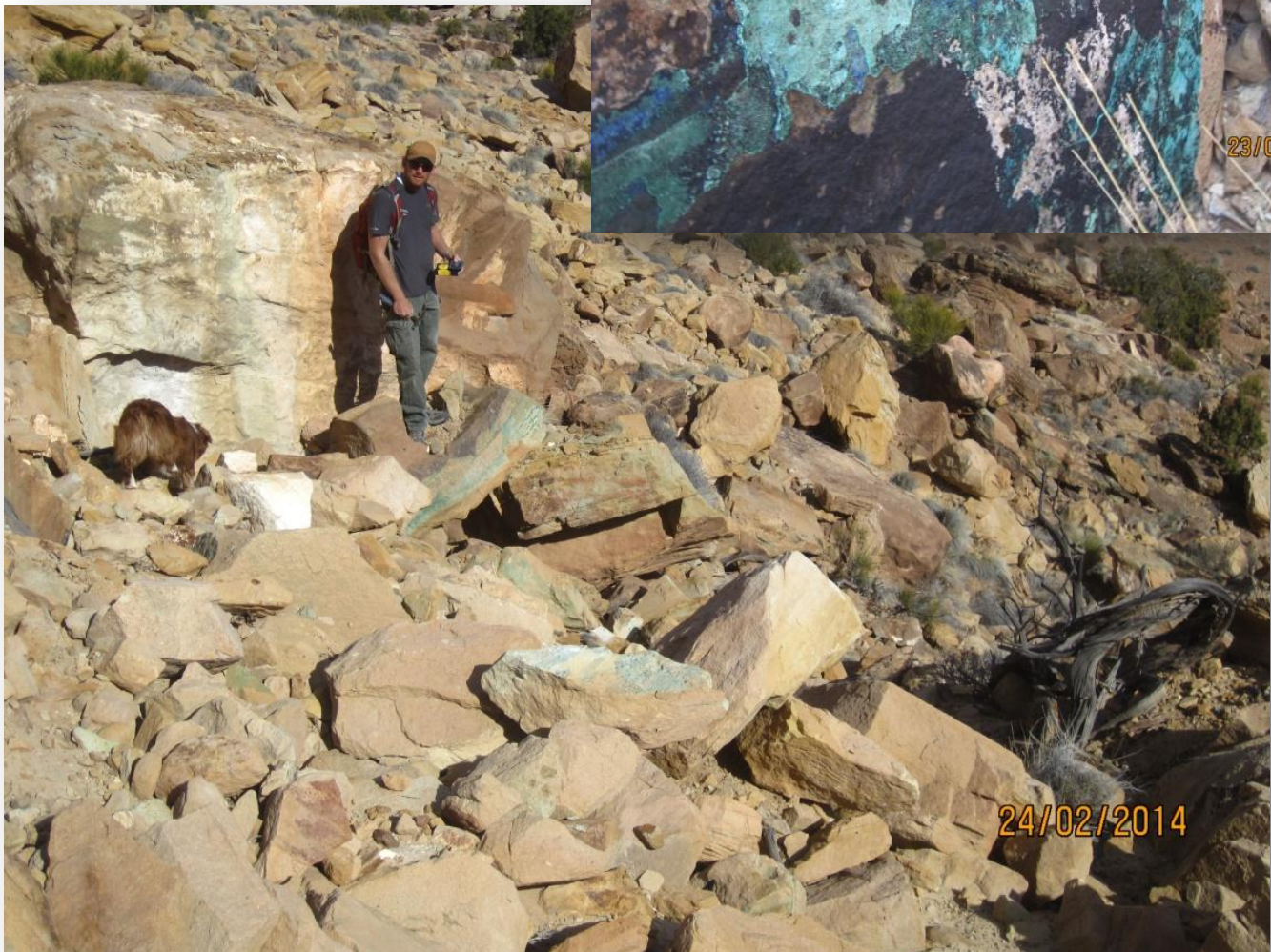
Photo of mineralisation near Harrison Prospect. ( Inset photo is copper filling fracture).
