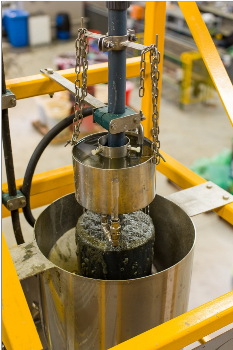
Jameson flotation cell – (Xtrata Technologies) Second beneficiation pilot plant campaign, 1:2000 scale
