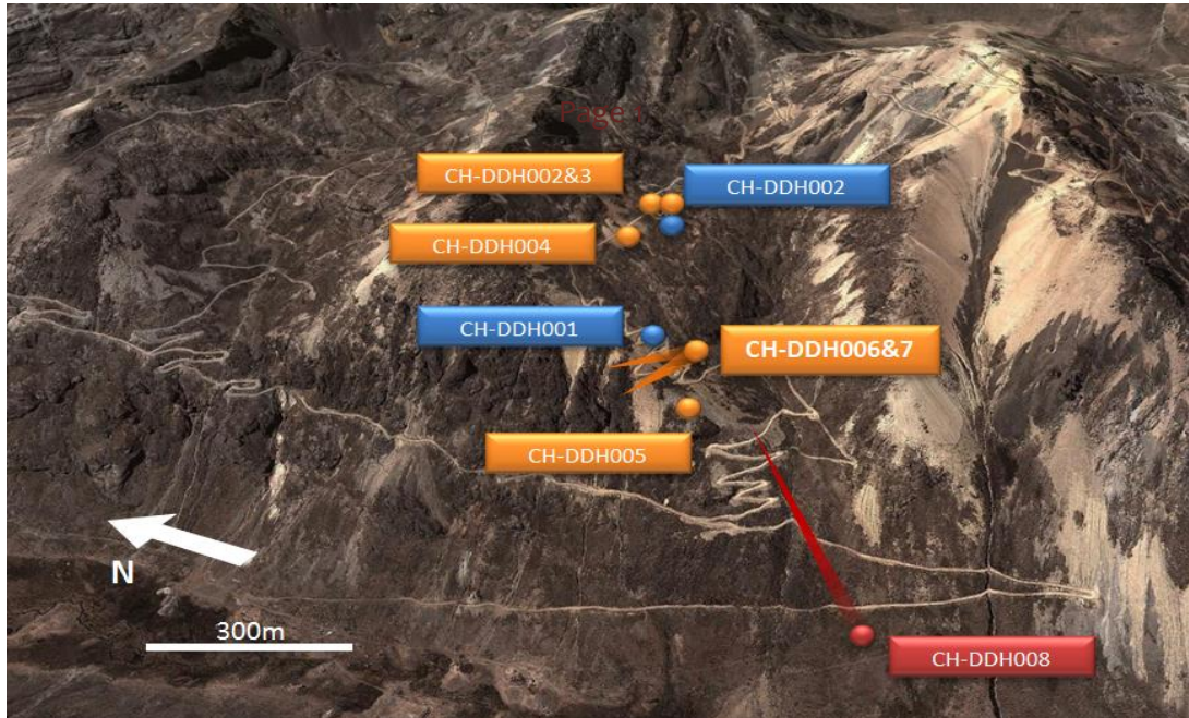
Figure 3: 3D terrain image of the Chanape Project area looking towards the ENE. Drill hole CH-DDH008 is positioned SW of CH-DDH001. This hole tested the possible south west extension of the known porphyry in CH-DDH001.
