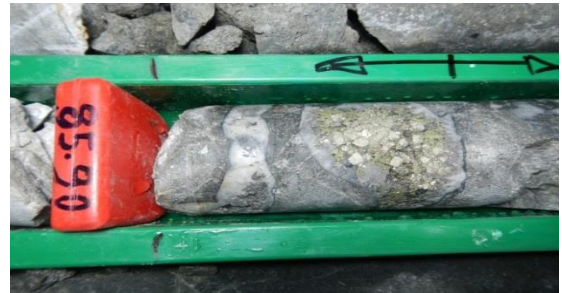
Figure 2: Chalcopyrite/pyrite/qtz vein at 85.9m (CH-DDH006)
