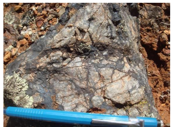
Figure 13. Supergene manganese matrix infill of quartz breccia at Pier Dam
