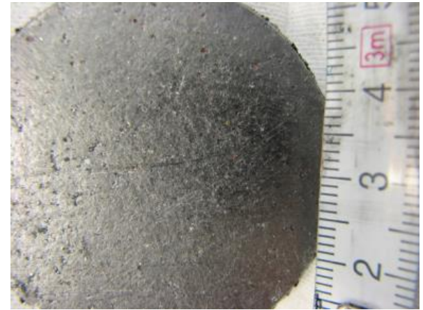
Graphite foil produced from Kibaran flake graphite
