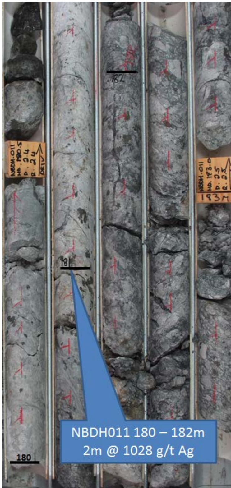
Figure 6 – Intense massive, disseminated and stringer sulphide mineralisation, with native silver and copper both visually, XRF and assay confirmed.
