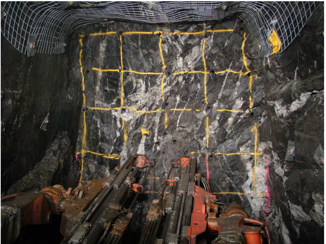
Jumbo drilling 1100S_5901405.0N face that returned 3.0m grading 9.7 g/t Au (view south) [often where the main eastern reef narrows (left of photo) the best grades present]
