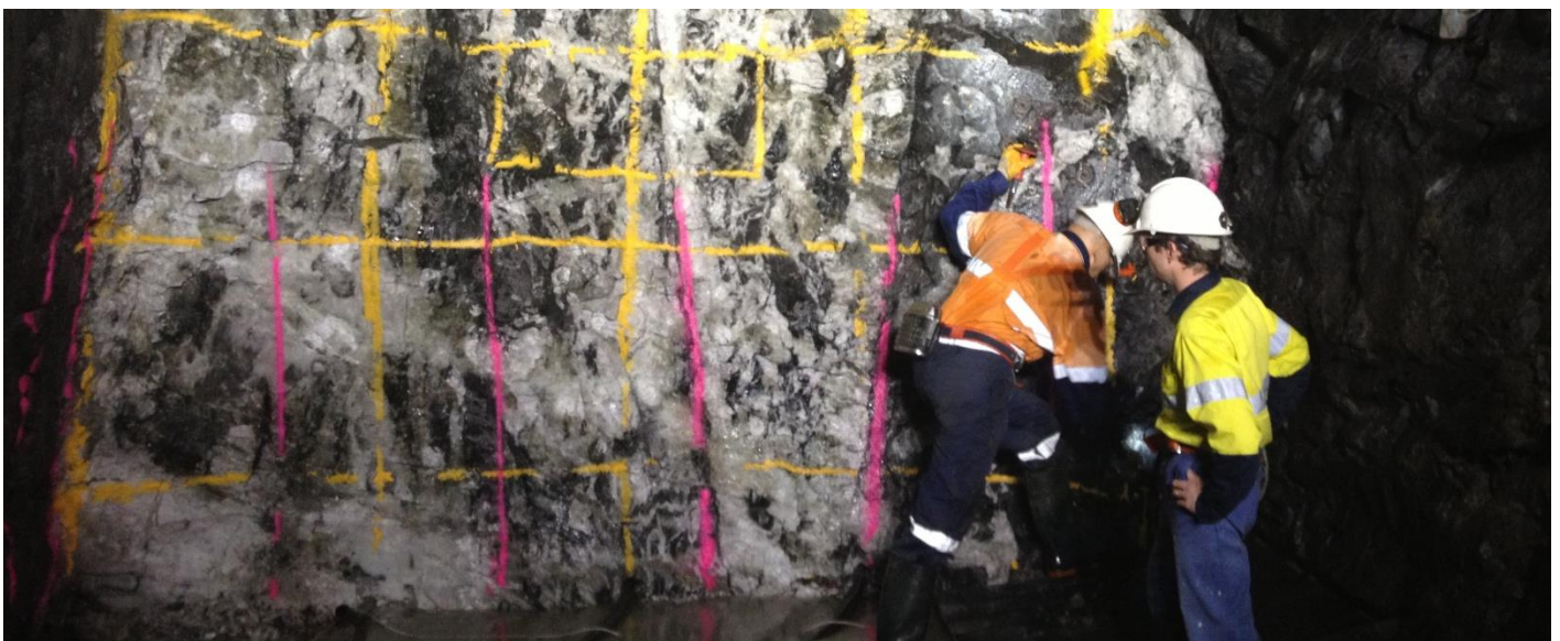
Underground mine development face marked up for channel sampling (pink lines) and blast hole pattern (yellow lines)
