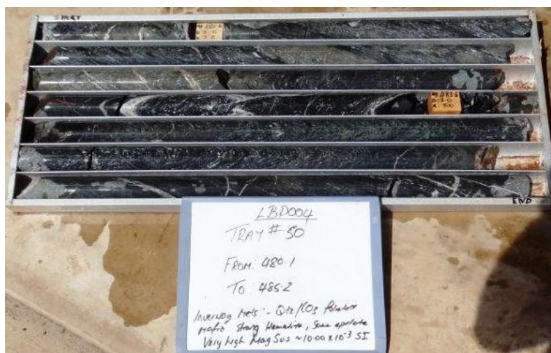
Figure 5. Strong magnetometer readings towards base of hole in foliated quartz-carbonated mafic rock.
